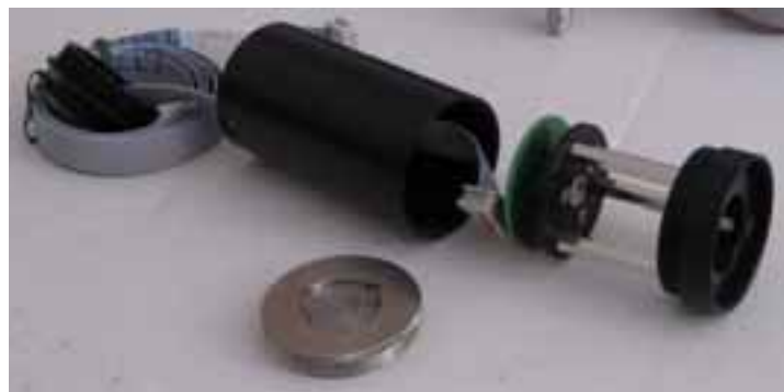
Fig. 3. A two-axis sensor with narrow FOV and elevated precision.
