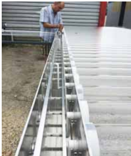
Fig. 7: Rolling mechanism stress tests
