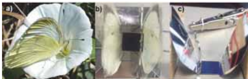
Fig. 9: (a) The cabbage white butterfly (photographed by Tina Pilipović, permission for use granted). (b) Top view of wings positioned in V shape with 1cm x 1cm solar cell at base of wings. (c) Side view of reflective film in shape of wings also positioned in V shape.
