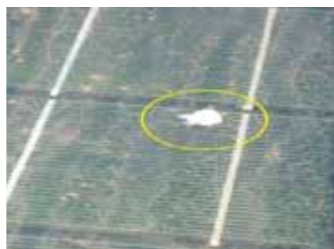
Fig. 6: Fauna droppings on the panels - 1 st August 2014
