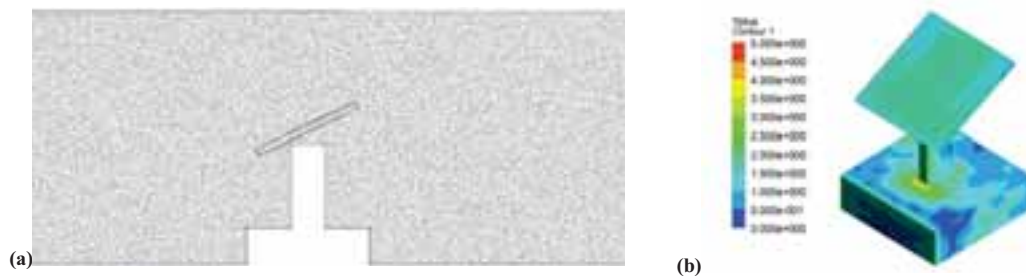
Fig. 5: (a) Polyhedral mesh at the middle plane of the domain; (b) Y-plus at the heliostat plate is \sim 2 .
