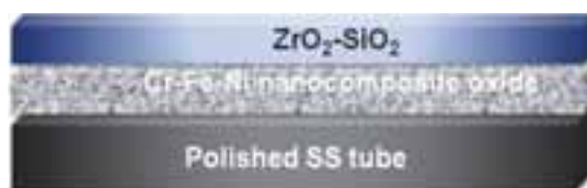
Figure 1. Schematic diagram of the Cr-Fe-Ni oxides / ZrO 2 -SiO 2 composite oxide layer deposited on stainless steel tube
