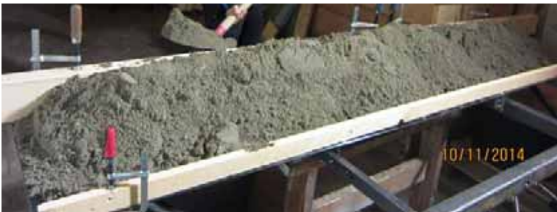
Fig. 14: Glass stripe of 4mm thickness loaded with sand simulating the maximum expected wind loads.
