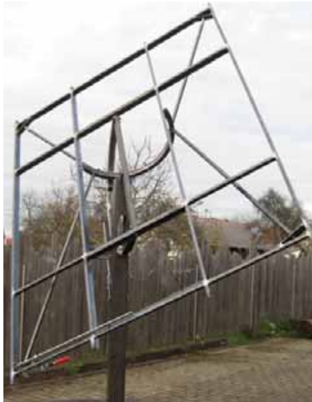
Fig. 10: First frame work mirror support structure with too high flexibility regarding bending about its diagonals.
