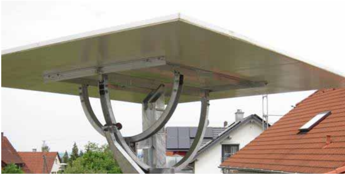
Fig. 4: First rim drive heliostat with sandwich mirror panel
