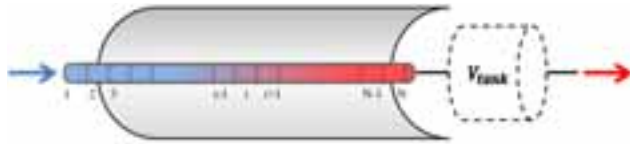
Fig. 2: one-dimensional discretization of a PTC (with a fictive tank connected to the outlet for the simplified model)
