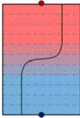
Fig. 4: one-dimensional finite-volume method for modeling a thermocline storage
