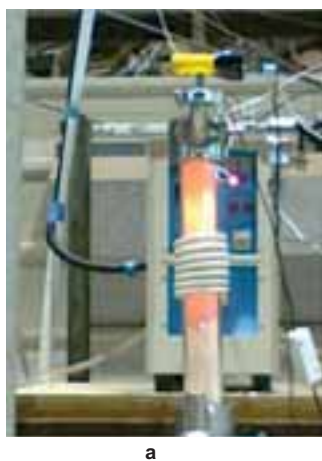
Fig.6: IH vacuum reactor: (a) photo of the Induction Heating (IH) vacuum reactor during operation; (b) principle schemes of non-solar IH setup (temperature in reaction crucibles 1400-1800°C and on deposit sites from 200°C to 1500°C)
