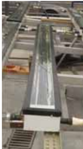
Figure 4: CPC designed and built.
