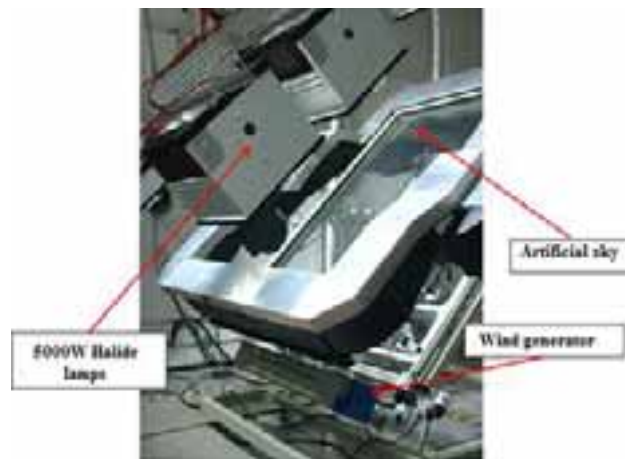
Figure 1 – Solar simulator, front view
