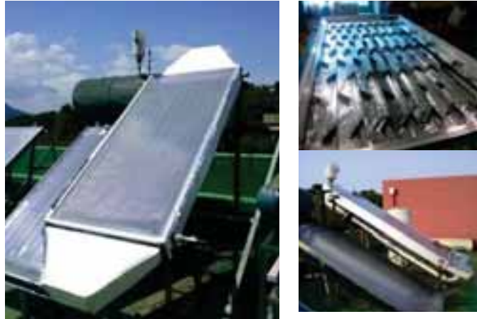
Fig. 1: Actual feature of hybrid solar collector for experiment
