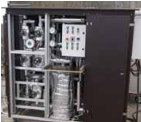
Figure 5: Test rig for conditioning of pressurized water and the data acquisition unit
