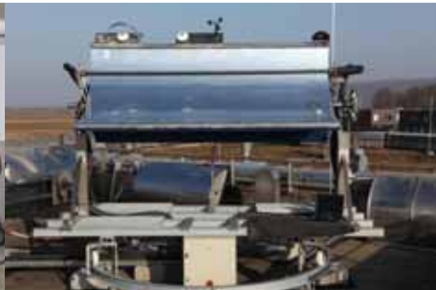
Figure 6: Biaxial rotating test platform with an installed reference collector
