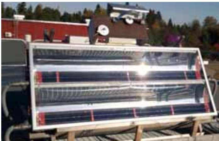
Fig. 1: Solarus C-PVT collector and solar radiation sensor
