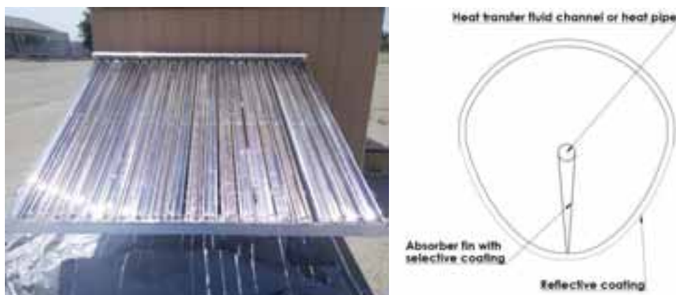
Fig 5: a) The ICPC 3.5 m 2 prototype, with full 1900mm length tube, front view. b) The cross section of the original ICPC prototype design.
