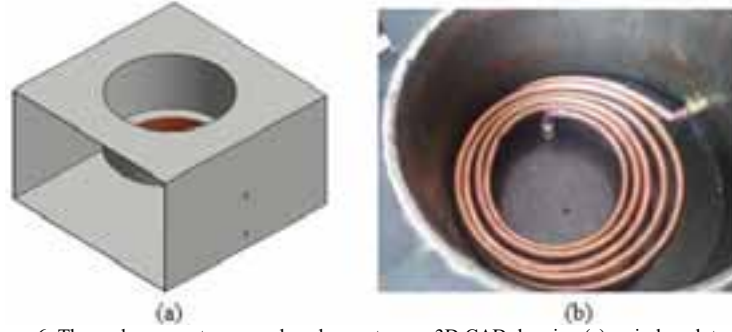
Figure 6: Thermal energy storage and cooker: cut-away 3D CAD drawing (a), spiral cook top (b)
