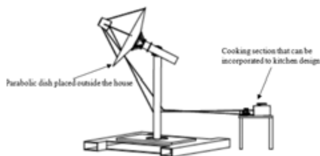
Figure 2: Complete CAD drawing of the experimental setup
