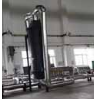
Fig.1 Photo of packed-bed TES unit
