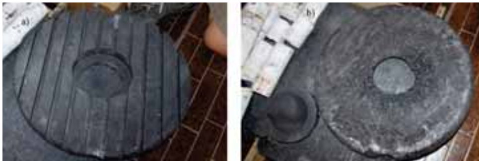
Fig. 7: Lower graphite disc after the charge of the TES unit. a) Face of the lower disc pointing inside the crucible in direct contact with the glass melt. b) Face of the lower disc pointing outside of the crucible in contact with the atmosphere.
