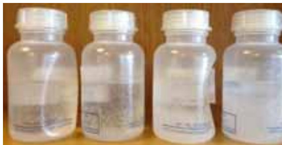
Fig. 5: 5 cm salt water mixtures after 129 days supercooling, 46%, 45%, 42%, 40% water samples from left to right
