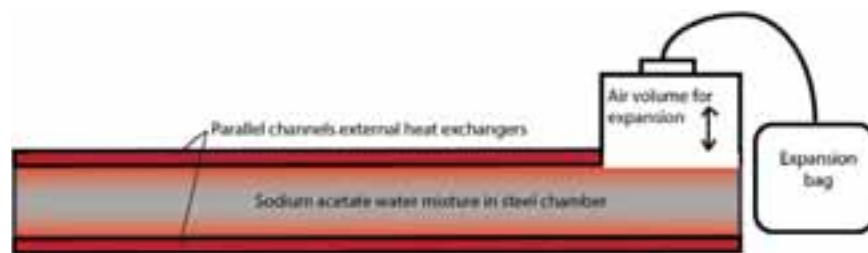
Fig. 10: Diagram of the prototype module (Dannemand et al., 2015)
