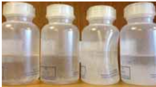
Fig. 4: 4 cm salt water mixtures after 126 days supercooling, 46%, 45%, 42%, 40% water samples from left to right
