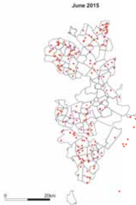
Fig. 1: PV systems in Canberra which are actively reporting their power output every five minutes to PVOutput.org, before being ingested into the Regional PV Simulation System. The black lines are the boundaries of Canberra suburbs
