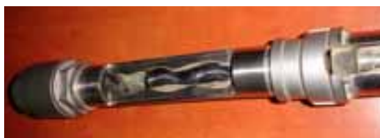
Fig. 2: Example helical rotor pump end commonly used for solar water pumping.
