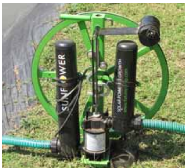
Fig. 3: The Futurepump piston water pumping system manufactured in India retails for US$400 with the PV module.
