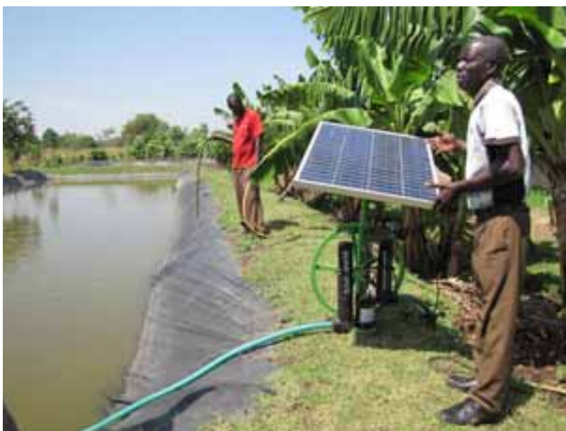
Fig. 8: Mr. Joshua Okundi with his Futurepump PVWP, used to recirculate water for a tilapia pond for oxygenation and also to irrigate a banana grove. The farm is located near Kendu Bay on Lake Victoria in Kenya.
