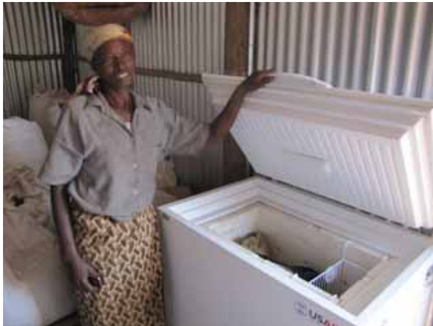
Fig. 9: Satisfied Ngorika dairy farmer is happy with the Solar FMC and is actually exceeding recommended design cooling capacity by successfully cooling 40 liters of evening milk overnight.
