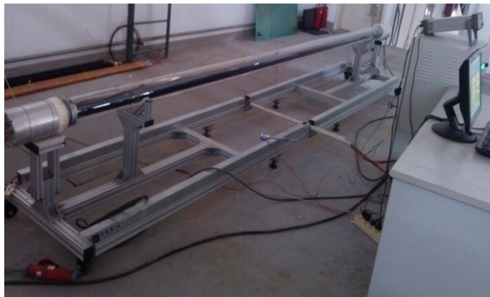
Fig. 3 Receiver heat loss test stand at IEECAS
