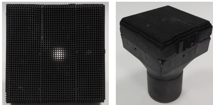
Fig. 3: Left, frontal photograph of the absorber aperture plane (square lateral size is 125 mm). Right, three-dimensional view of the complete receiver, composed of the absorber plus a cup-shaped air collecting manifold
