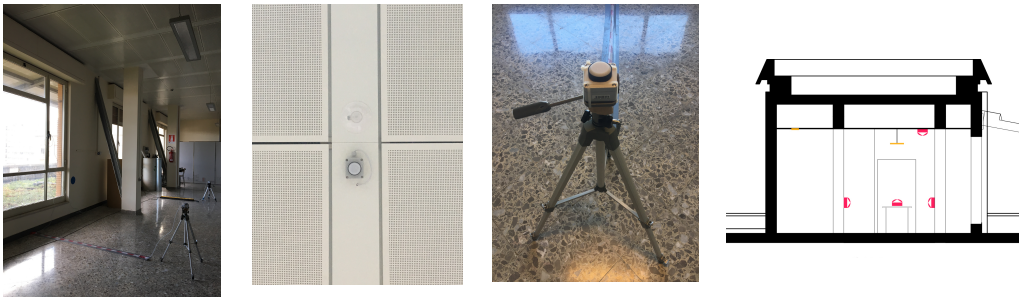
Fig. 1: Some pictures of the laboratory, of the sensors used to measure indoor illuminance and the section with their location.
