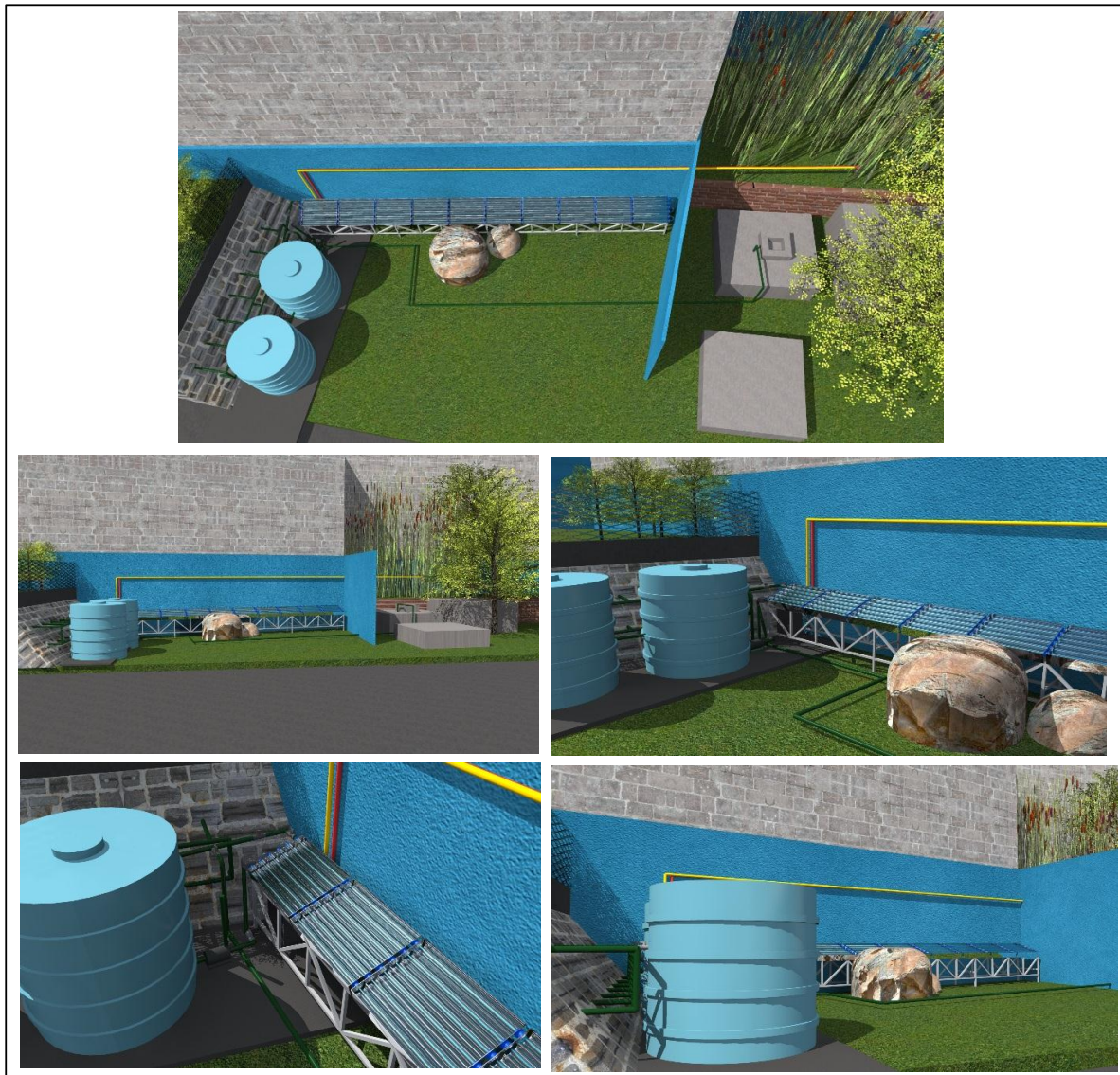
Fig. 7b: Digital sketch of the photocatalytic treatment system
