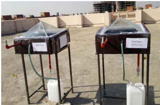
Fig. 8: Design development and study of solar distillation stills with different absorber coatings
