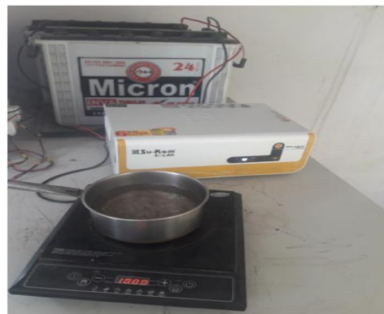
Fig. 11: Developed solar PV induction cooker
