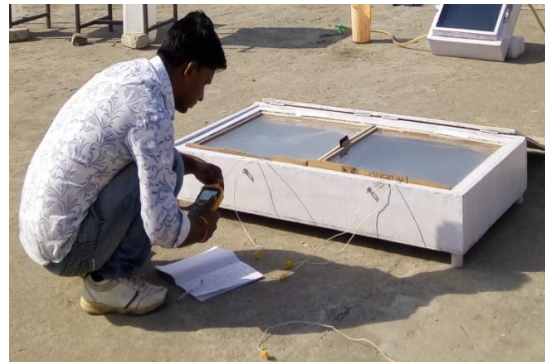
Fig. 9 Developed large size solar cooker/solar hot case
