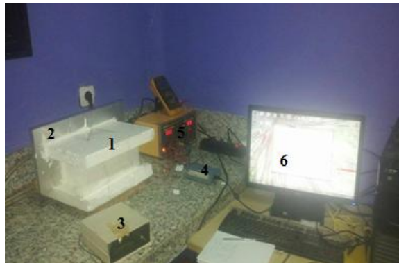
Fig. 1: Experimental setup. 1) The enclosure cavity. 2) The cold wall. 3) Temperature regulator. 4) Data acquisition, 5) Heating system, 6) Computer.
