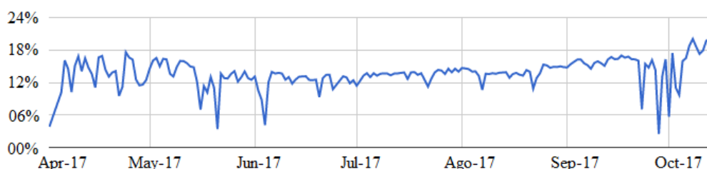
Fig. 10: Curve of daily capacity factor values observed on 34 kWp grid-connected PV system from April to October 2017.
