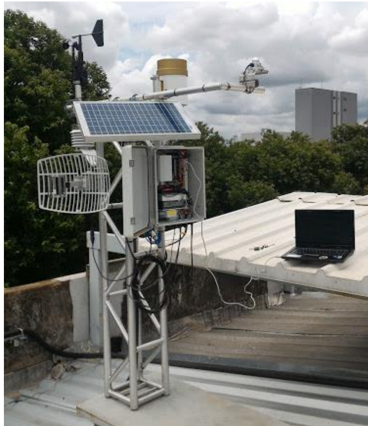
Fig. 6: Local weather station installed alongside the 34 kWp grid-connected PV system at UFG (Goiania, Brazil).
