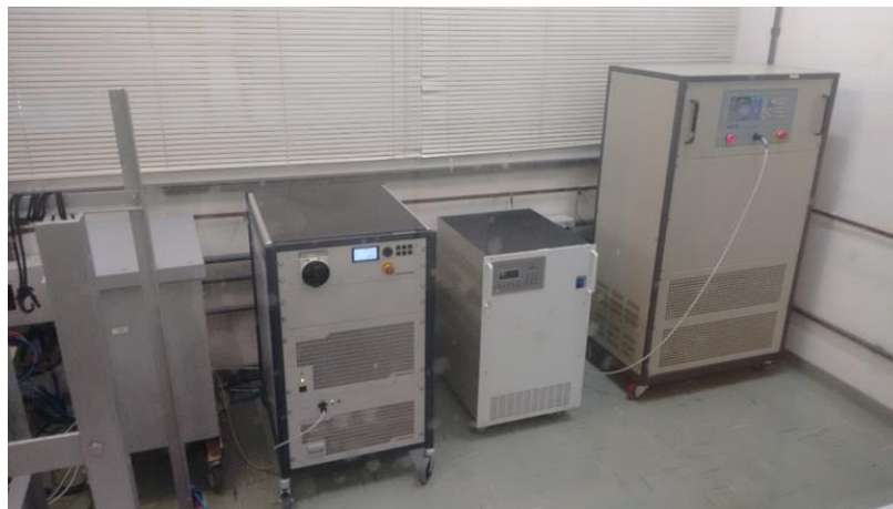
Fig. 5: LSF String Inverter test equipment. From left to right: S.A.S DC power source, grid simulator AC power source, and RLC load bank.
