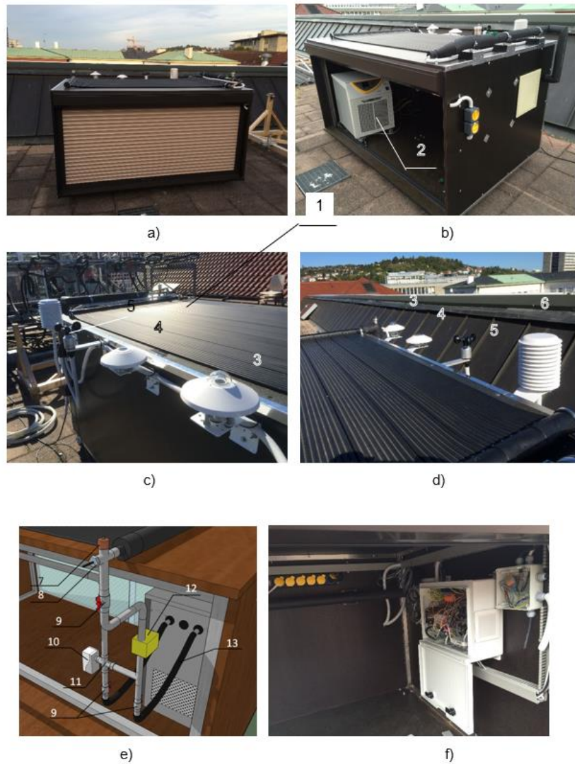
Fig. 4: HIL test bench: a) general view closed, b) general view open, c) and d) weather station, e) hydraulic system, f) electric control box
