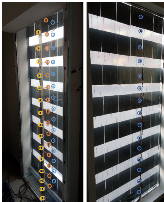
Figure 3 Thermocouples are placed on four layers on the DSF-PV (Left) and on the IGU-PV (Right).
