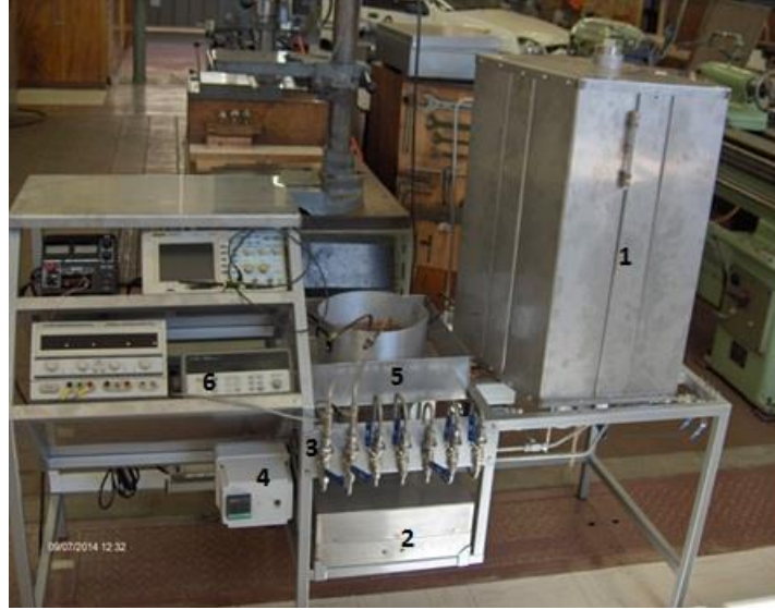
Figure 2: Photograph of experimental setup showing the main components. (1) Insulated storage tank (2) Electrical heater with copper spiral coil (3) Control valves (4) PID temperature controller (5) Discharging coil (6) Datalogger
