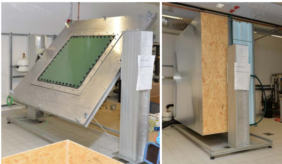
Figure 5: Test rig for practical testing of multi-layered wall structures in Chemnitz, enamelled and sealed wall segment (left), pivoting wall cut-out with thermal insulation and cladding panel in the vertical position during the test (right)
