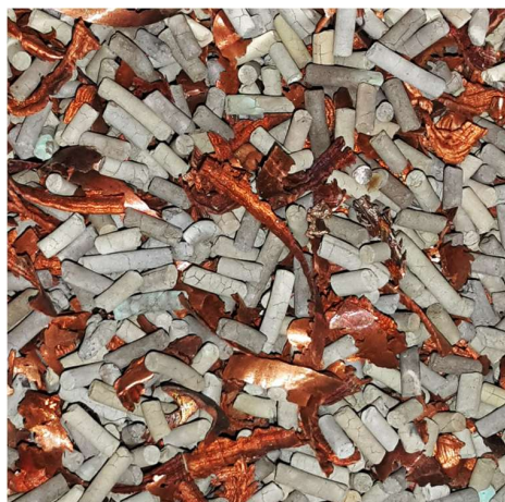
Fig. S4: A mixed packed bed loading of 13X-Cl and Cu-turnings
