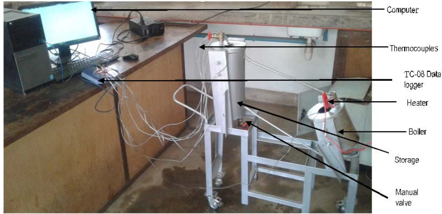
Fig. 2: A self circulating system consisting of a storage tank and a boiler. Sunflower oil was used in the boiler and the three types of oil where put in the storage tank one after the other. The storage was filled with each type of oil and this got heated in the boiler and thereby charging the storage.
