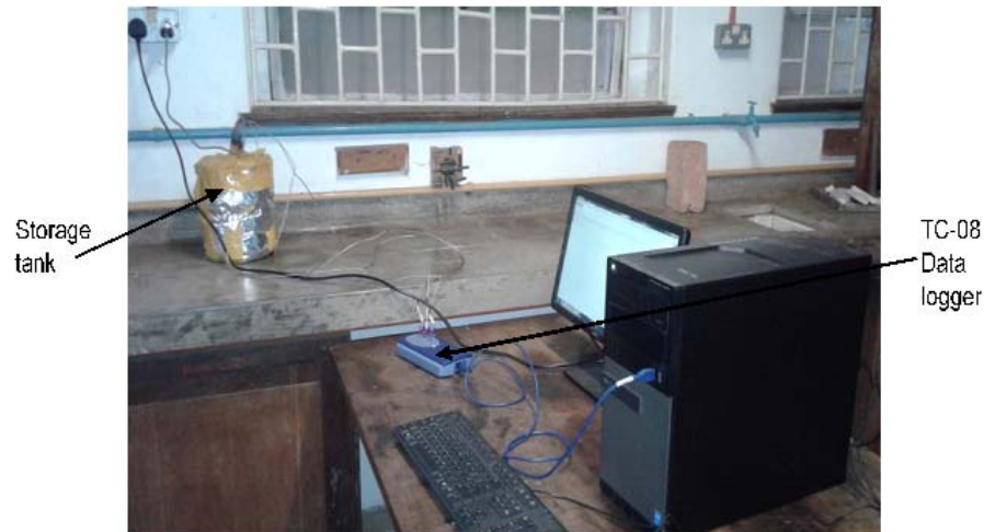
Fig. 1: Showing the experimental setup. The oil is heated in an insulated tank and thermocouples connected to a data logger and a computer were used to monitor and record the temperature during heating and cooling.
