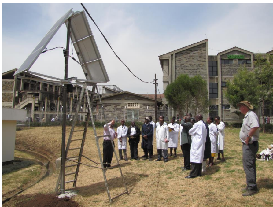
Fig. 5. FMC PV array (510 Wp) with unique East-West fixed tracking array under test at Egerton University Dairy Science Unit.
