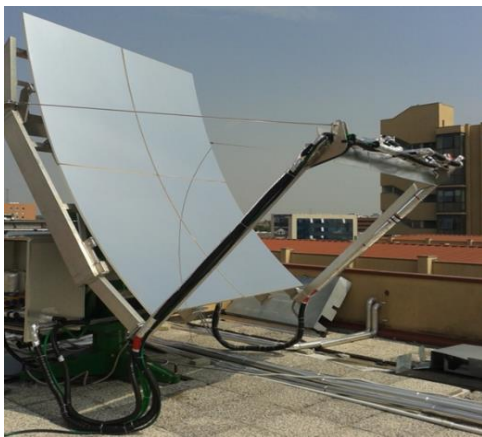
Figure 1. Asymmetrical parabolic trough linear solar concentrator installed in the Solar Energy Conversion Lab of the University of Padova.
