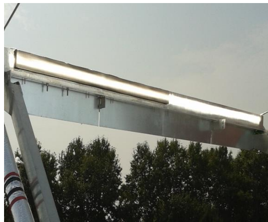
Figure 2. Bar-and-plate flat receiver arranged on the support bar of the collector under concentrated solar radiation during a test run.
