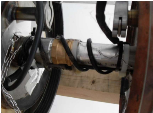
Fig. 15. Tracer on the connection pipe between the modules
