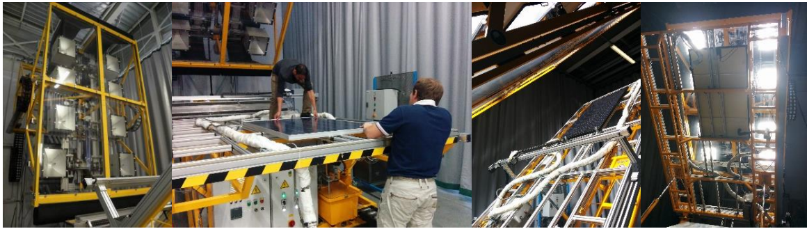
Fig. 2: Pictures of the artificial sunlight test bench
