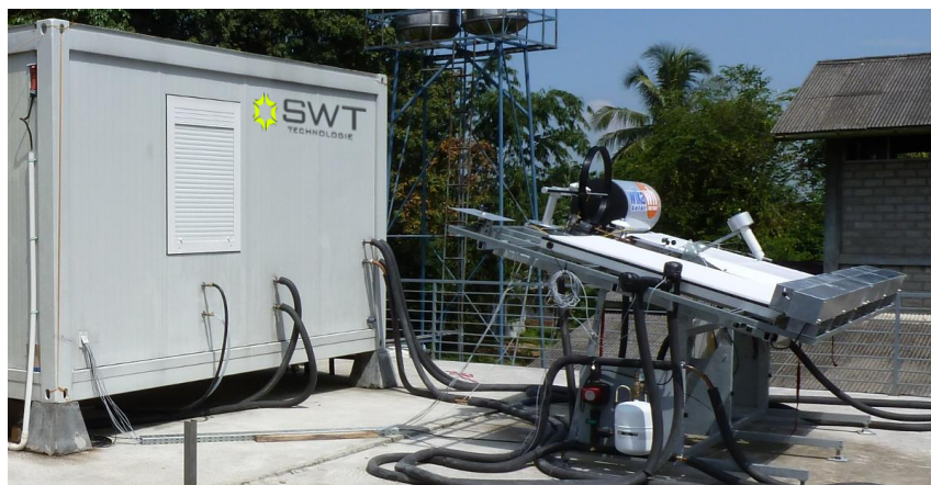
Fig. 4: Picture of the newly designed test rig for thermal performance tests of solar thermal systems and collectors
