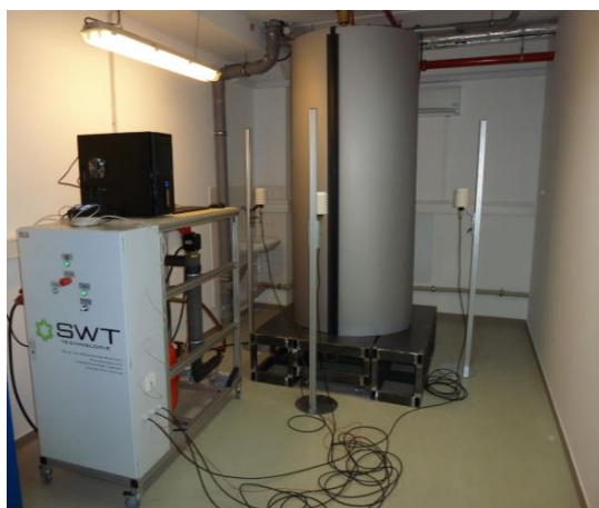
Fig. 5: Picture of the handy and mobile test facility for the determination of the heat loss rate of hot water stores
