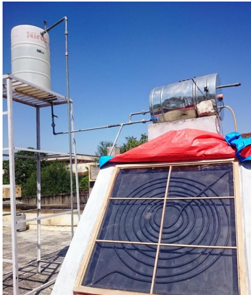
Fig. 1: Building material housing solar water heater (BMSWH)
