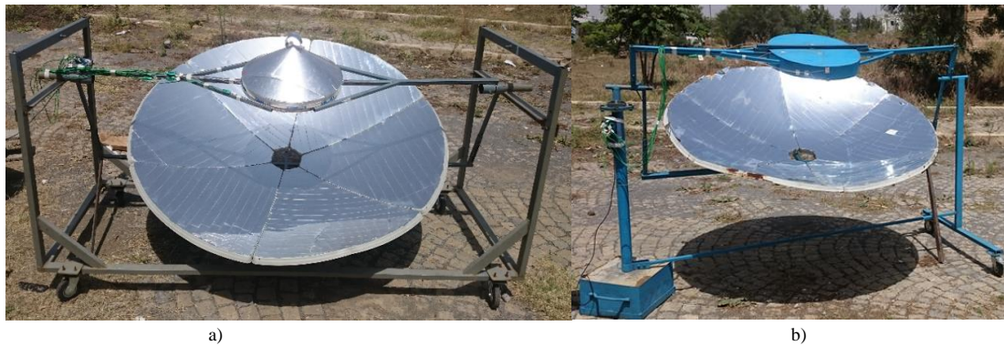
Figure 3: the direct solar fryer model a) with continuous heating-baking mode b) with alternative heating-baking mode
