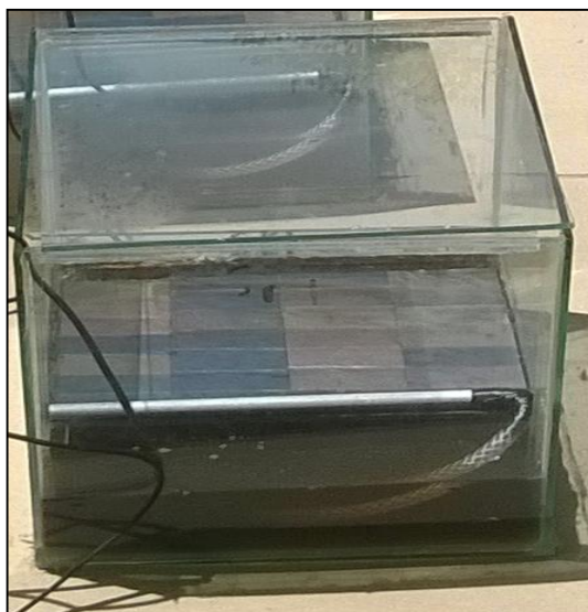
Plate 2: Fabricated photo catalytic effluent treatment unit
