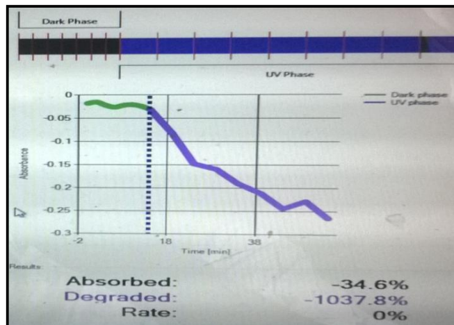
Plate 6: Degradation of methylene Blue with titanium plate anodised at 180 volts for 120 seconds and pigmented
