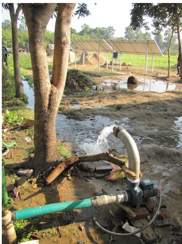
Fig. 4: Flood irrigation via a surface centrifugal solar water pump managed by Phattu Tharu of Bangadhi, Bardiya.
