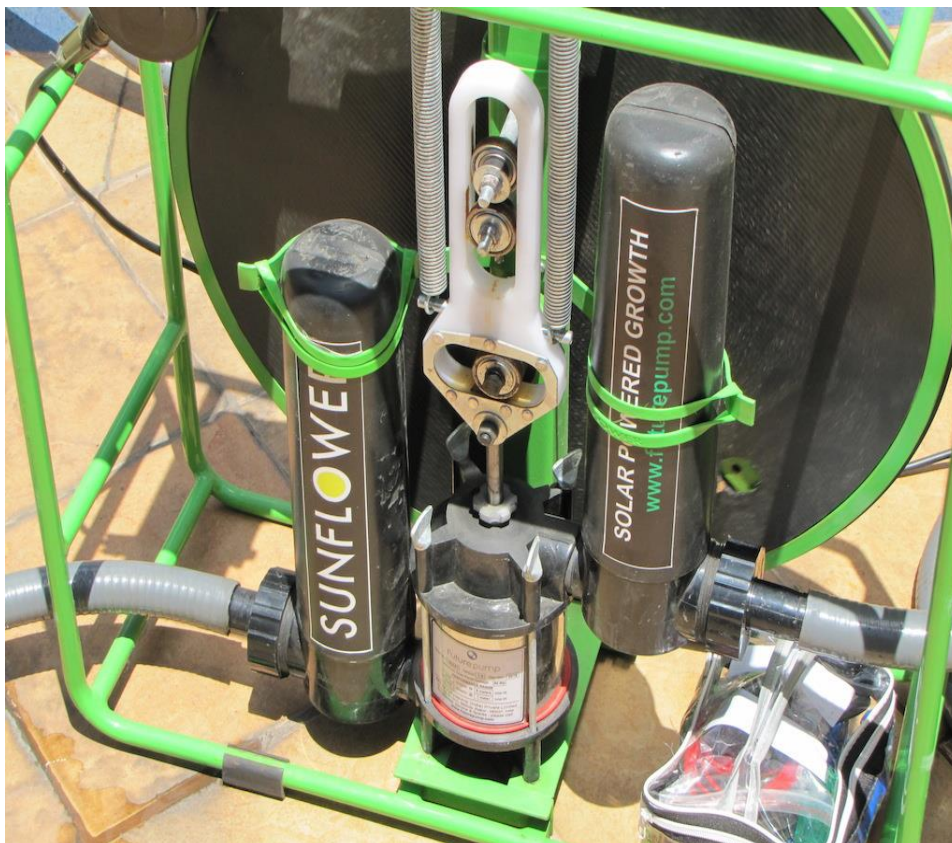
Fig. 2: Futurepump SunFlower (SF1) is a micro-size piston pump for small-farm irrigation. To reduce cost and complexity, it uses a two-speed manual transmission instead of an electronic controller, and manual solar tracking. Photo: Winrock International Kenya.
