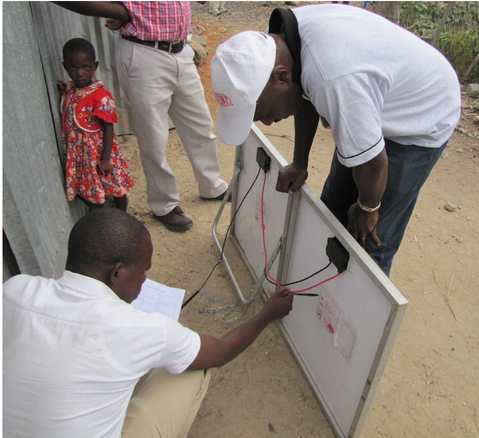
Fig. 4: Winrock technicians inspecting two Ubink PV modules made in Kenya for the Machakos solar diaphragm pump system. The farmer brings her PV modules in at night for security reasons.
