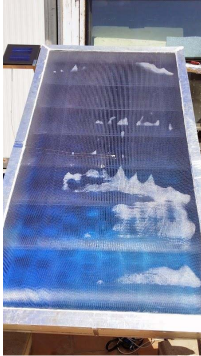
Fig. 8 Condensation phenomenon observed in a preliminary prototype
