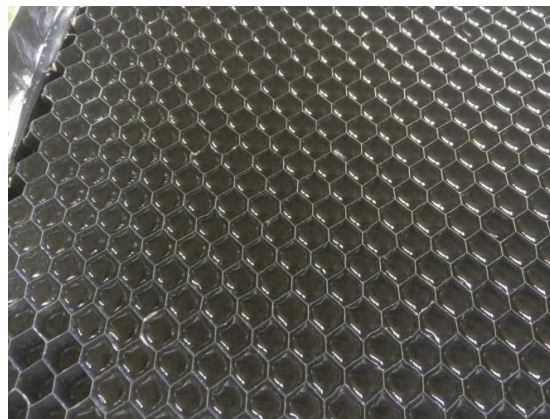
Fig. 2: Honeycomb filled with PCM
