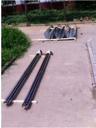
Figure 5 – Side-By-Side Stagnation Test Setup
