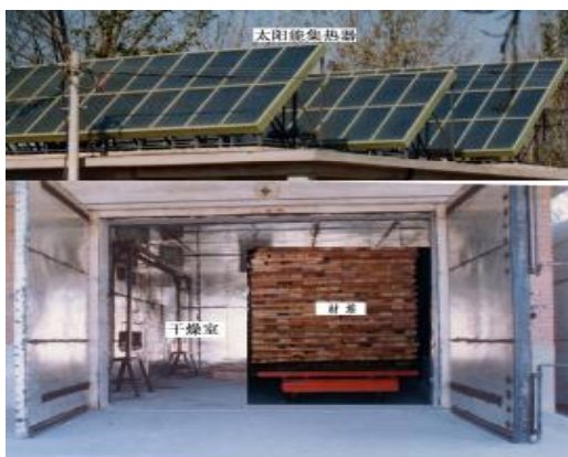
Fig. 7: Solar wood drying
